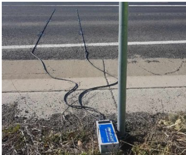
Example of pneumatic road tubes
