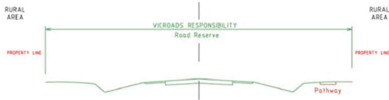
Figure 4 – Demarcation Arrangements for Typical Rural Arterial Roads
