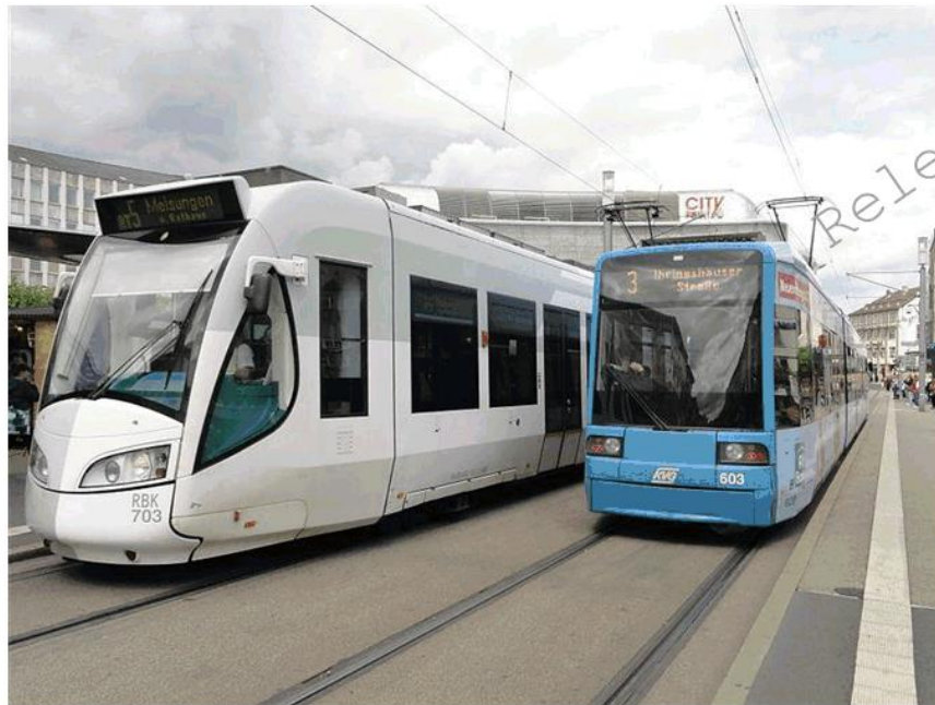
Figure 23 RegioTram Kassel dual voltage DC/AC Alstom Regio-Citadis next to a KVG Bombardier Flexity Classic tram at Königsplatz
