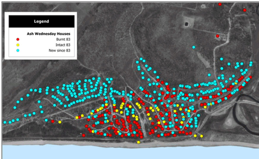
Figure 21 Dwellings in Fairhaven following Ash Wednesday fire Red dots indicate houses that were burnt during the Ash Wednesday fire of 1983 and yellow dots indicate houses that remained intact. Blue dots represent houses that have been built since 1983, which are in addition to the houses re-built on the red-dot sites.
