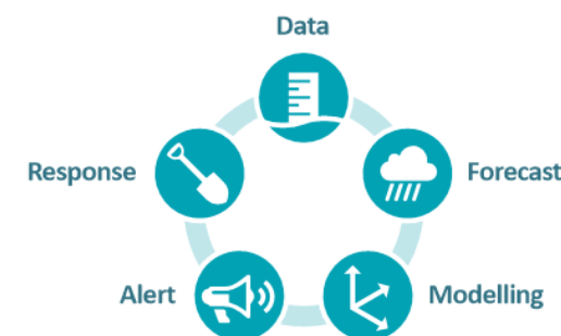
Figure 2. Elements of a Total Flood Warning System. (Source – Victorian Floodplain Management Strategy)
