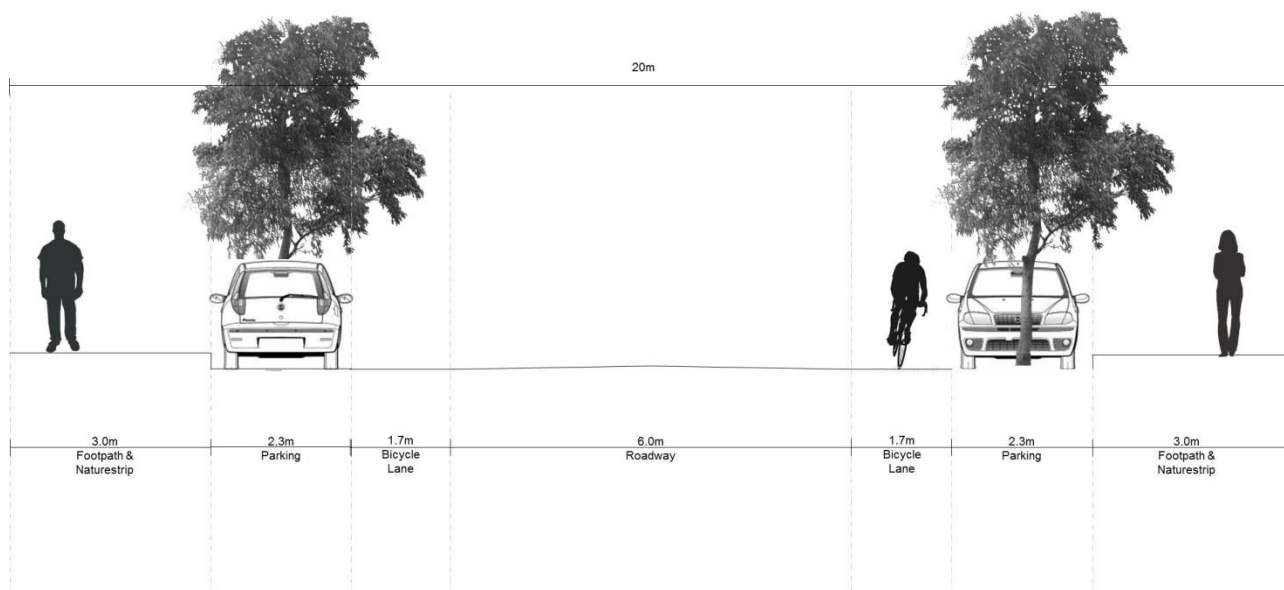
Figure 4: Cycle Friendly Road Cross Section (shown as Figure 35 in the O'Brien Report)
