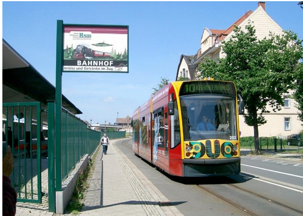
Figure 22 A Nordhausen 'DUO' Combino on the track linking the urban tramway, where it is electrically powered via overhead wires, and the HSB (Harzer Schmalspurbahn) rural railway, where it is powered by an on board diesel engine
