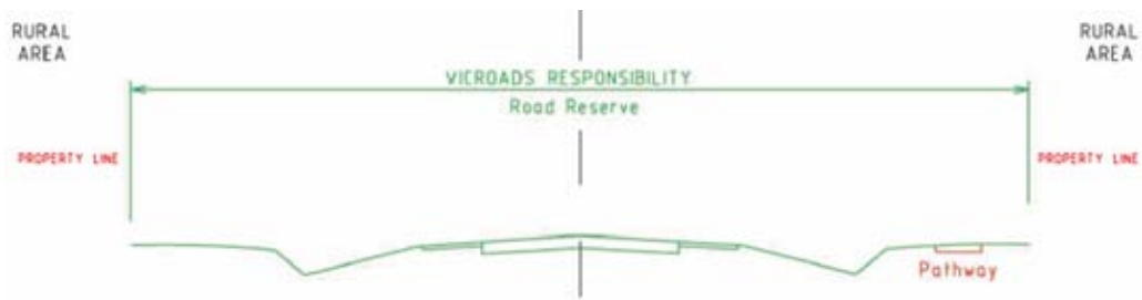
Figure 4 – Demarcation Arrangements for Typical Rural Arterial Roads
