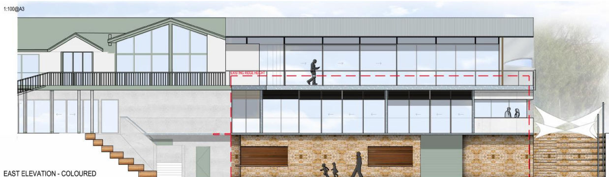
Figure 2 – East elevation which shows existing building and height of the existing building to be demolished
