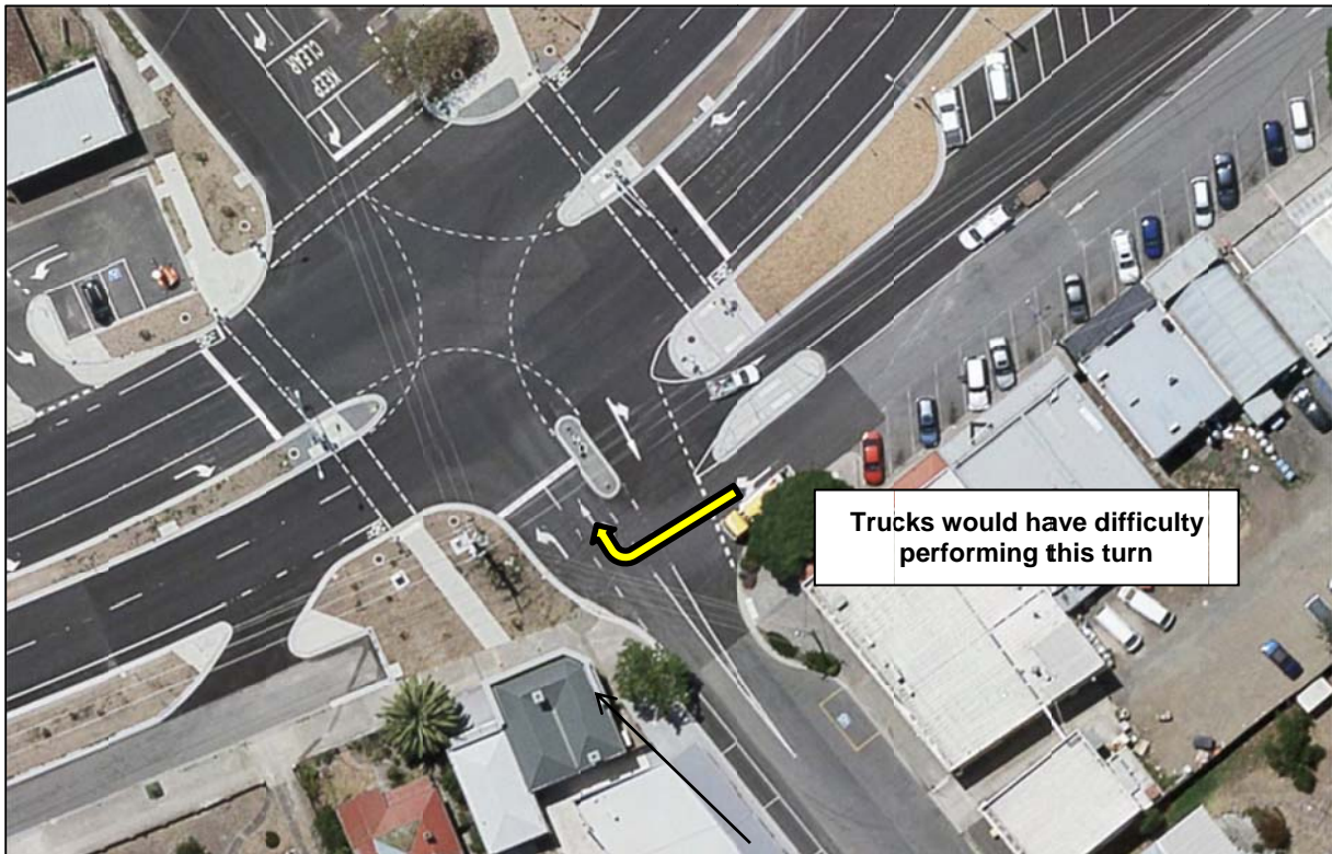
Figure 20: Princes Hwy / Hesse Street – difficult truck access
